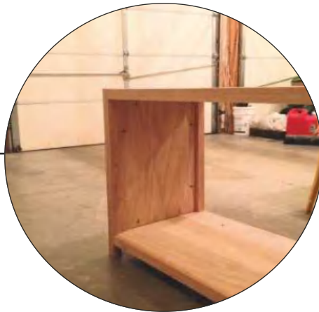
STEP 11. The divider panels can then be cut and secured with pocket jig screws
